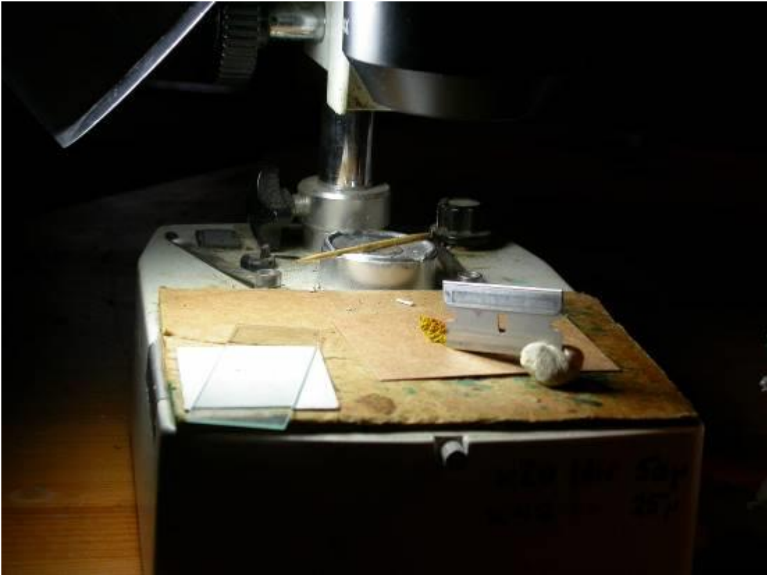
Sectioning a Xanthoria thallus (hand removed from razor, which is now held in place with tack). Note razor at shallow angle, anchored in card behind the cut, the blade will now be drawn gently backwards (towards right edge of photograph) with tip of razor still in contact with card. Also note light coming in from the left, and microscope slide conveniently close on stage of dissecting 'scope' (a droplet of mountant is already in middle of slide ready to receive the section).
