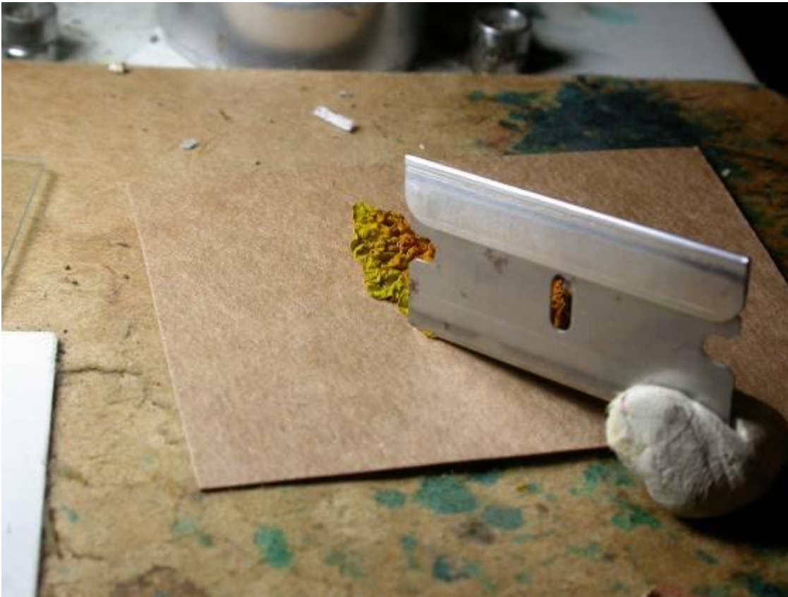
Closer view of sectioning, the thin sliver to be examined will be pared off on left side of blade.
